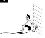
Plug each blower into a 115 volt electrical outlet. Make sure the outlet has either a SLO-BLO 20 AMP fuse or 30 AMP fuse circuit. The blower should be the only thing plugged into that circuit. If two blows required they must be on separate circuits.
